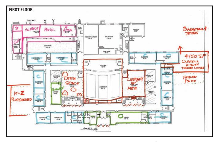
The existing classroom areas would be reconfigured to provide new rooms ranging in size from 725 s. f. to 850 s. f. with the majority being in the 750-800 s. f. range. The north courtyard would be enclosed to provide a library which would be at the heart of the school. The south courtyard would be landscaped as a protected outdoor play area.
